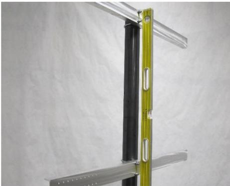
Hold a level on centerline as shown. Note bubble. Now move level to outer end of channel next to brackets. The bubble on the level must read the same; this will ensure that the panels are in plane. Now tighten the U-Bolts. If the channels are not in plane then you will have a twist to your panel(s).
