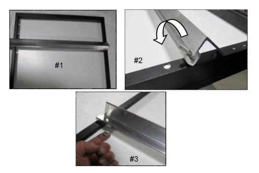
**For T-Slot Rails**: Lay T-Slot rails across the short axis of the panel as shown in Photo #1.
